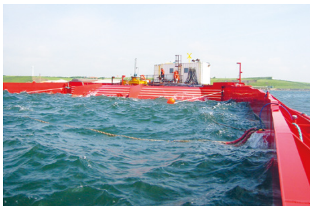
Wave Dragon overtopping wave energy converter (image courtesy of Wave Dragon).
