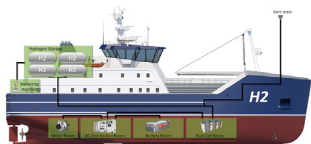
Layout of a conceptual hydrogen powered vessel (BMT)
