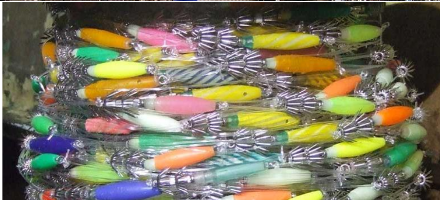
Figure 10 Deck of an Australian squid jigging vessel showing the multiple jigging machine arrangement showing arrangement of jigging machines (upper pic). A series of colourful squid jigs wound around a jigging machine drum (lower pic). Note the two rows of radially spaced barbless hooks on each jig.
