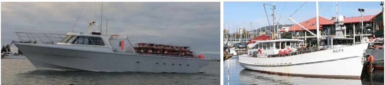
Figure 14. Two forms of cray boats; forward wheelhouse and planning hull (left), aft wheelhouse and displacement hull (right)
