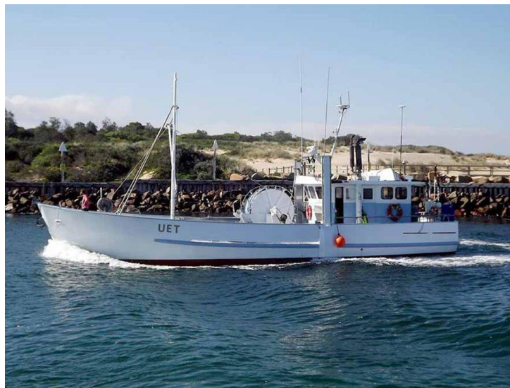
Figure 5. FV Erin Jay - a Commonwealth shark gillnetter fishing out of Lakes Entrance. Note the large drum on the foredeck to hold the long net. (Source: Erin Jay - www.leftrade.com.au ).
