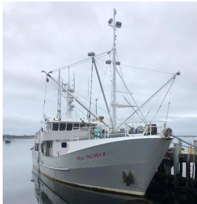
Figure 9. FV Del Richey 2, a Commonwealth Southern Squid Jig fishery vessel (20m aft wheelhouse vessel) (Source: Andrew Sullivan)
